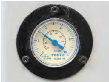
4 - Pressure when Pressing The optimum pressure for the deformation of the blank is 3 bar.
