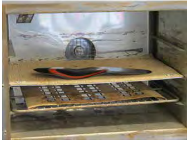
1 - Heating of the Blank Place the carbon blank in a forced air oven at 120°C for 10 min.
