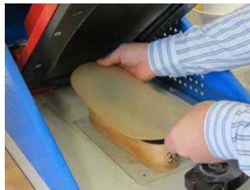
5 - Place the Silicone Film Cover the heated blank with a silicone film, so it does not stick on the machine.
