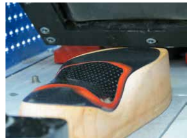
6 - Cool After 15 min of cooling, the blank has assumed the shape of the last. Now remove the silicone sheets.
