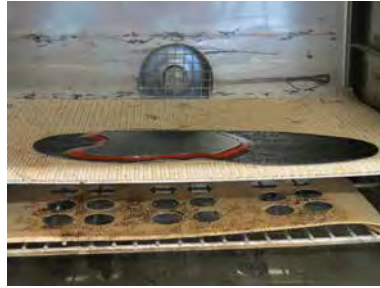
2 - Blank after Heating The heated blank is now flat and can be deformed again in the heated state.
