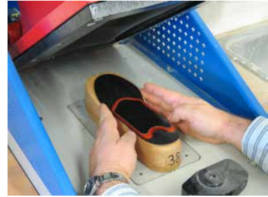
3 - Deforming in the Last Press Place the blank on the appropriate last of your choice.
